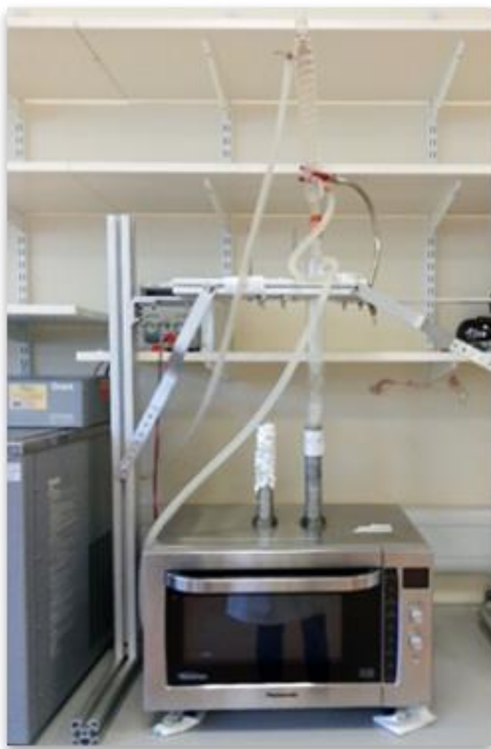
Figure S1. Lab-designed microwave system used for the microwave-assisted extractions.
