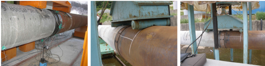
Figure 5. Three-point bending test of mechanical joint of a steel pile and a concrete pile [9].
