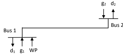
Figure 4.6. Two-bus power system
