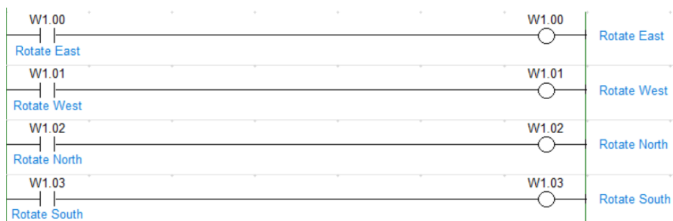
Figure 3.15 Outputs ladder section
