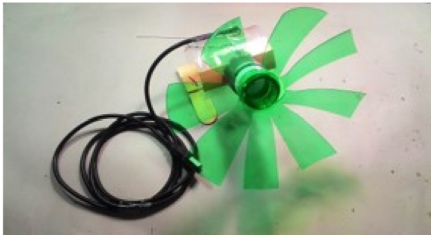
Figure 4.16: Using a plastic bottle to create a fan using a motor.
