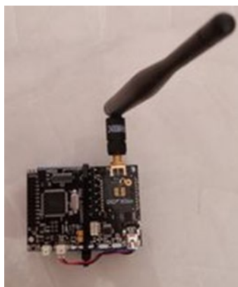
Figure 14. Wasp-mote device equipped with the 802.15.4 module.
