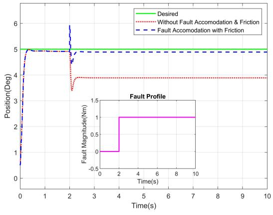
Fig 16. Position tracking of waist joint of a robot manipulator with abrupt fault profile.
