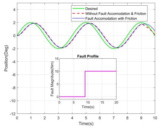
Fig 13. Sinusoidal response of shoulder joint of a robot manipulator with abrupt fault profile.
