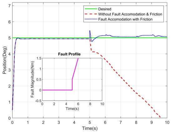
Fig 17. Position tracking of elbow joint of a robot manipulator with incipient fault profile.
