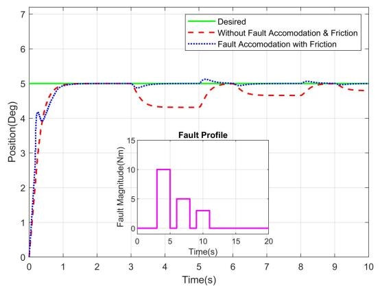
Fig 11. Position tracking of shoulder joint of a robot manipulator with intermittent fault profile.
