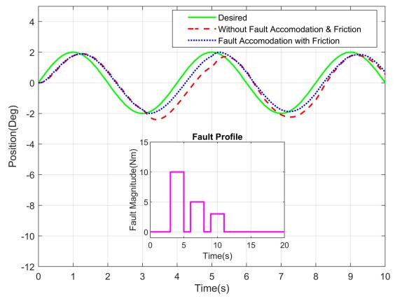
Fig 12. Sinusoidal response of elbow joint of a robot manipulator with intermittent fault profile. https://doi.org/10.1371/journal.pone.0256491.g012
