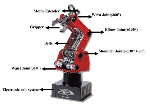
Fig 6. AUTAREP manipulator ED-7220C showing various joints with their Range Of Motion(ROM). https://doi.org/10.1371/journal.pone.0256491.g006
