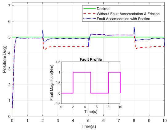
Fig 18. Position tracking of shoulder joint of a robot manipulator with intermittent fault profile.
