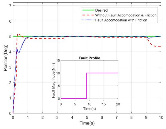
Fig 10. Position tracking of elbow joint of a robot manipulator with abrupt fault profile.
