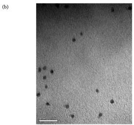
**Figure 1.** (a) Structure of chlorpromazine hydrochloride in planar (left) and quasi-equatorial (right) conformations. The latter has been drawn to emphasize the boat conformation of the central six-ring. (b) Transmission electron micrograph of chlorpromazine hydrochloride aggregates obtained in an aqueous solution comprising 13.1 mM chlorpromazine hydrochloride and 36.0 mM zinc chloride. The scale bar corresponds to 50 nm.
