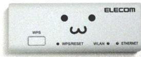
Figure 7. The compact wireless router (64×18×24mm) that was employed in mobile experiments with the Wireless Data Glove.
