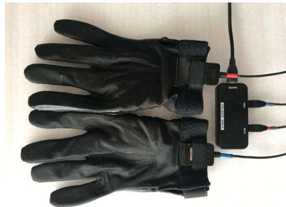
Figure 2. A pair of Yamaha Data Gloves wired to a 2-channel USB communication device.
