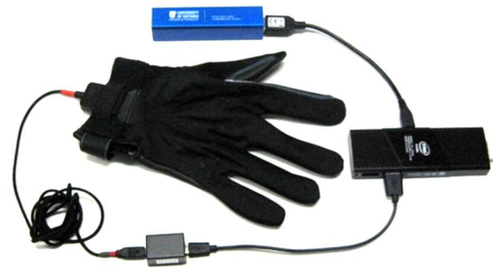
Figure 8. The wearable components of the wireless Data Glove set: the Data Glove in the middle, the USB2DG converter in the bottom, the Stick PC on the right, and the mobile battery on the top.
