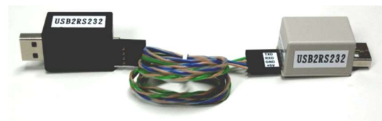
Figure 6. Two USB2RS232 converters wired together.
