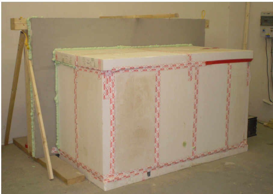
Fig. 1. Curtain walling test panel of the prefabricated wooden building structure.
