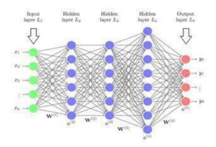
Figure 7. Simple Artificial Neural Network with Three Hidden Layers [11]
