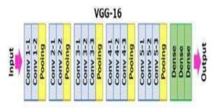
Figure 8. 3D VGG-16 Architecture [12]
