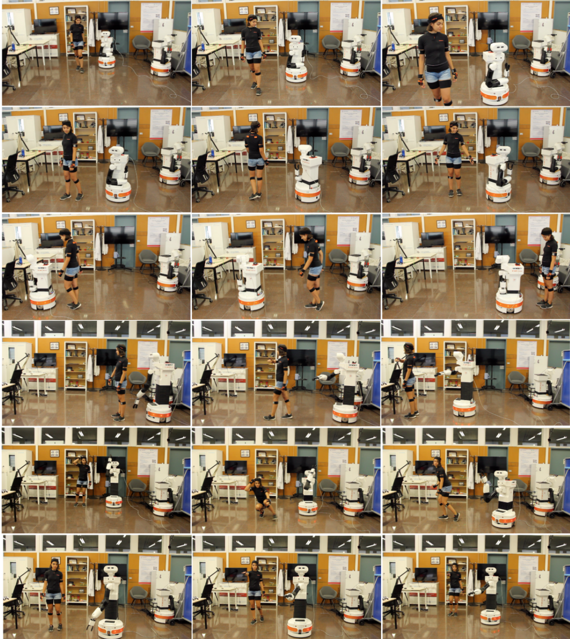
Figure 5.20: Several demonstrations of the mobile base motion transfer system performance with TIAGo. The robot accurately reproduces the walking motion of the human demonstrator. This includes forward and backward motions, and rotations. In some of the experiments, upper body motion is also transferred simultaneously.
