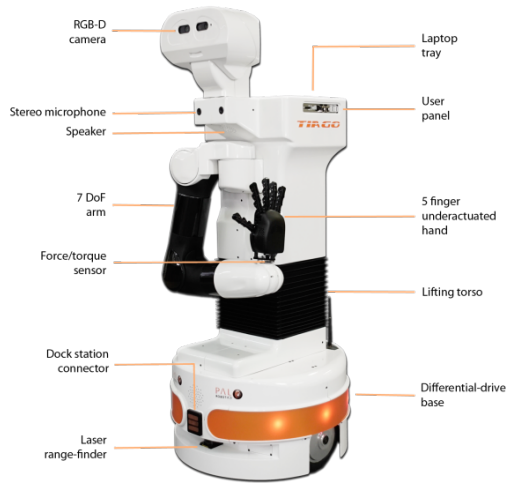
Figure 5.13: Overview of the main components of the TIAGo robot.
