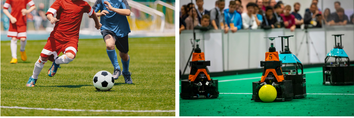
Figure 5.2: Humans and robots playing soccer. Due to differences in embodiment humans run and kick while robots roll and bump for accomplishing the same task.
