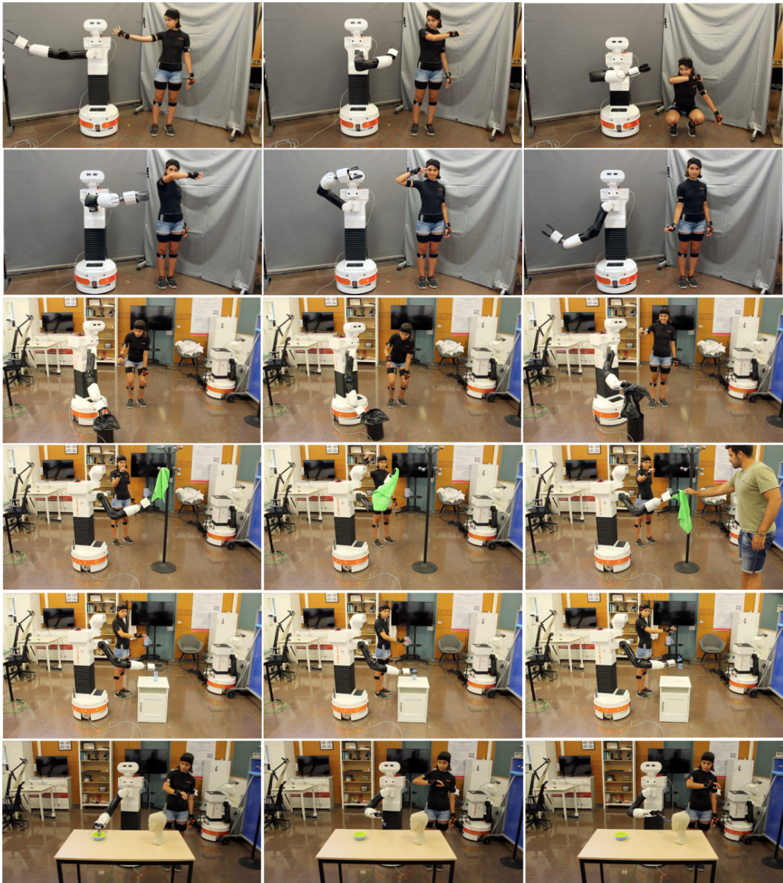
Figure 5.18: Several demonstrations of upper body motion transfer system performance. The robot accurately reproduces the movements of the human teacher. As we can see in some of the experiments depicted in this figure, our system opens the door for non-robotic experts to teach manipulation skills to a robot intuitively.
