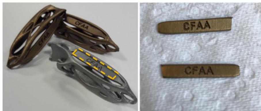
Figure 1. AlTiSiN coated specimens—Set 1.
