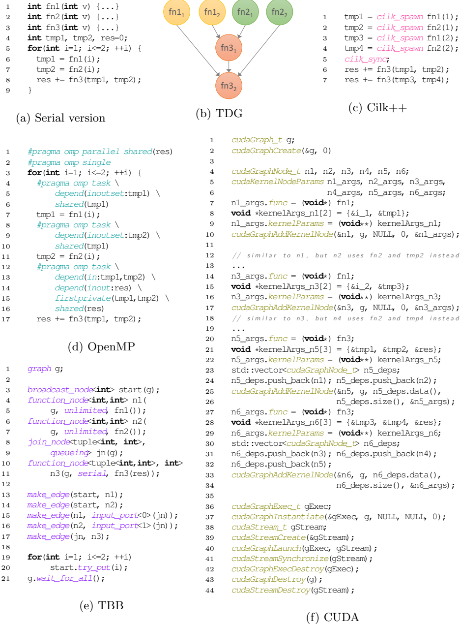
Fig. 4: TDG representation and high-level description of a simple code parallelized with different task-based programming models.
