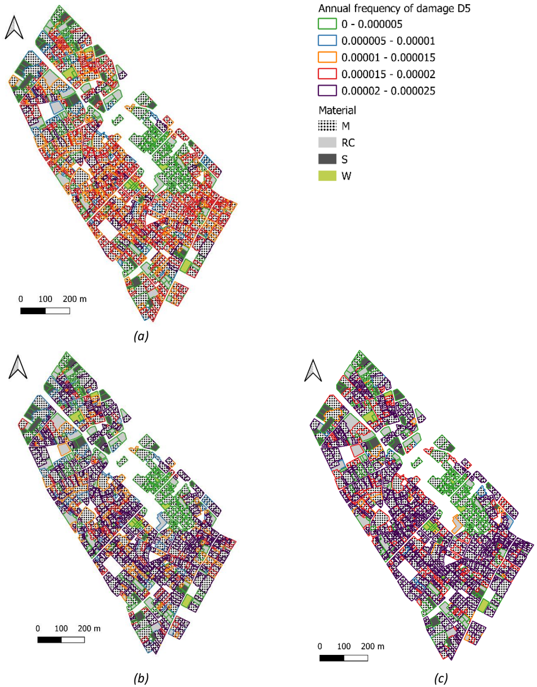
657 Figure 22. Seismic risk maps of the Gothic neighborhood of Ciutat Vella to cadastral plot scale. These maps show the seismic 658 risk and the main structural material of each residential building of the Gothic neighborhood of Ciutat Vella. The seismic 659 risk is in terms of annual frequency of damage D5, and this risk was obtained considering a seismic hazard curve truncated 660 to 475 years and the Lower (a), Best (b), and Upper (c) seismic vulnerabilities curves.
