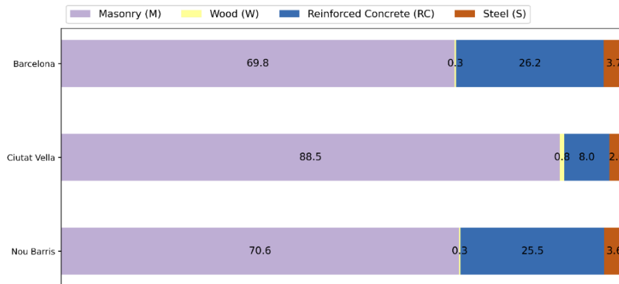
312 313 Figure 7. Distribution (%) of buildings by primary structural material (M-Masonry, S-Steel, RC-Reinforced Concrete, W- 314 Wood) for 69982 buildings in Barcelona, 5675 buildings in Ciutat Vella, and 6916 buildings in Nou Barris.
