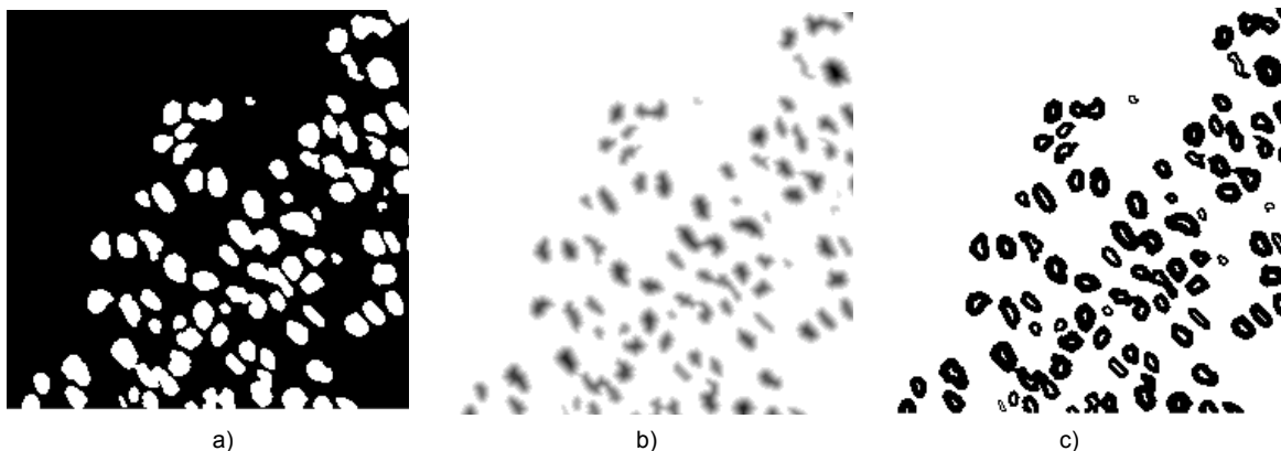
Figure 20: The left image represents the slice of a binarized prediction, the middle one the inverse of the result of applying the distance transformation, and the right one shows the markers for the watershed.
