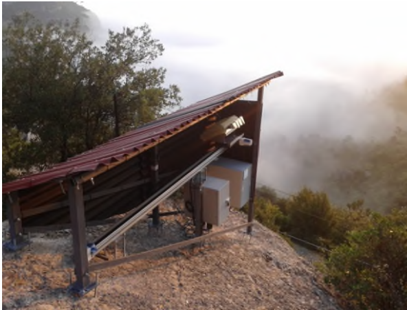
Figure 11. RiskSAR system placed at Pont de Guilleumes site with weatherproof cover for temporary use at short term.
