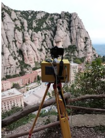
Figure 9. Data acquisition with the TLS equipment in Montserrat Monastery cliff.
