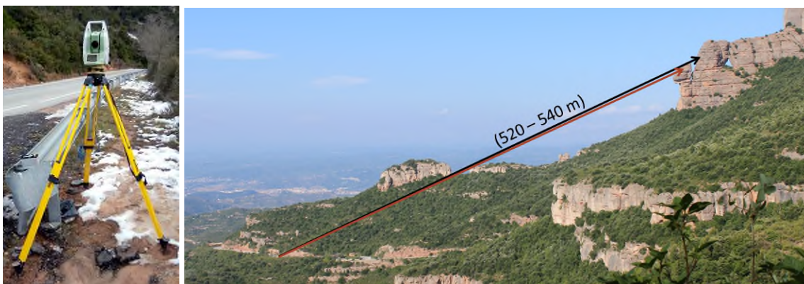
Figure 4. Leica TM30 Total Station used in Montserrat, and lateral view of the Cadireta and the base station (in the road).
