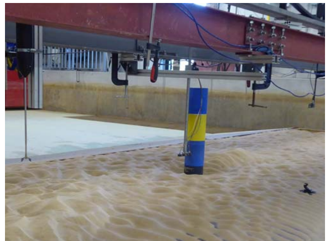
Fig. 12. Final state of the sand bed for current-only case (flow from left to right).
