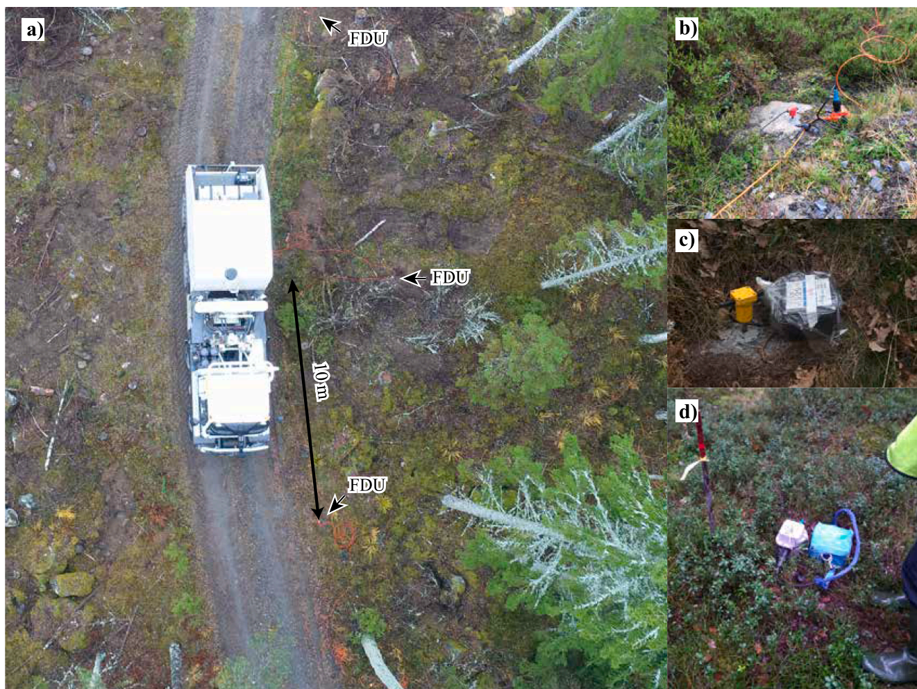
Fig. 3. Seismic source and various receiver types used during the Zinkgruvan acquisition (November 2018). (a) Aerial photo of the 32 t vibrator along profile P1. (b) SERCEL 428 cabled system, (c) CUBE wireless data recorders, and (d) Sercel UNITE wireless 1C recorders where possible geophones were planted in the bedrock to obtain higher S/N data.
