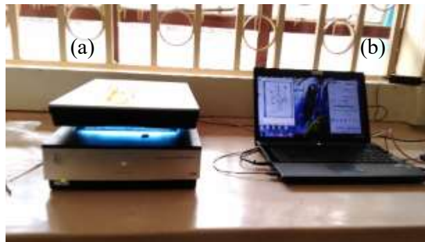
Figure 4.1: Scanning (a) and processing (b) of roots using Epson Expression 1680 Scanner.
