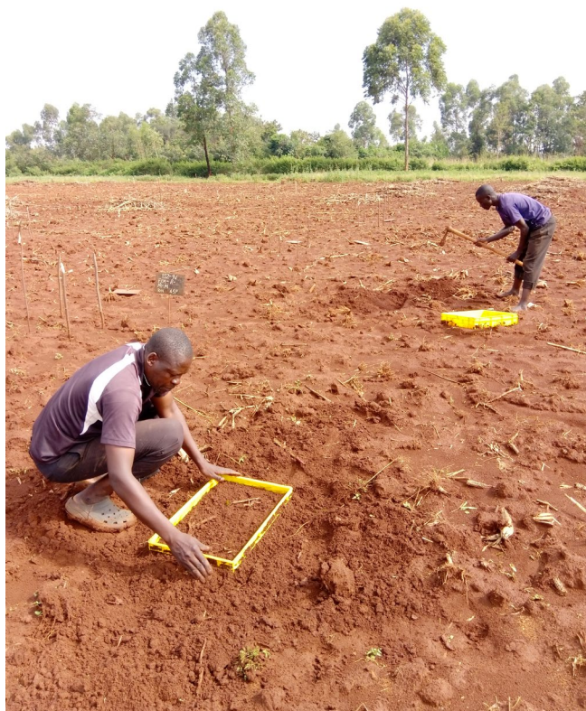
Plate 3. Installation of chamber bases and sampling of greenhouse gases under selected ISFM systems in INM3 (Photo: Peter Bolo/Alliance).
