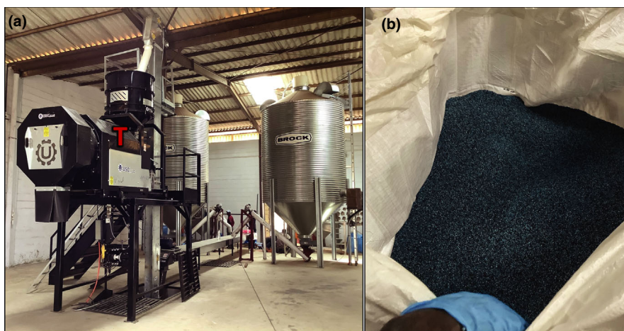
Fig. 2. Manufacturing facility in Kahone, Senegal where a seed treater (T) is used to coat roasted sorghum grains with a mixture of spore suspension, blue food colorant and a polymer (A). Biocontrol product temporarily stored in a 1-ton bag and ready to be packaged in 5 kg plastic bags (B).
