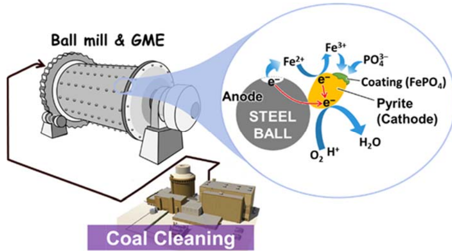
Fig. 1. A schematic diagram of galvanic microencapsulation (GME) in a ball mill containing steel ball media.
