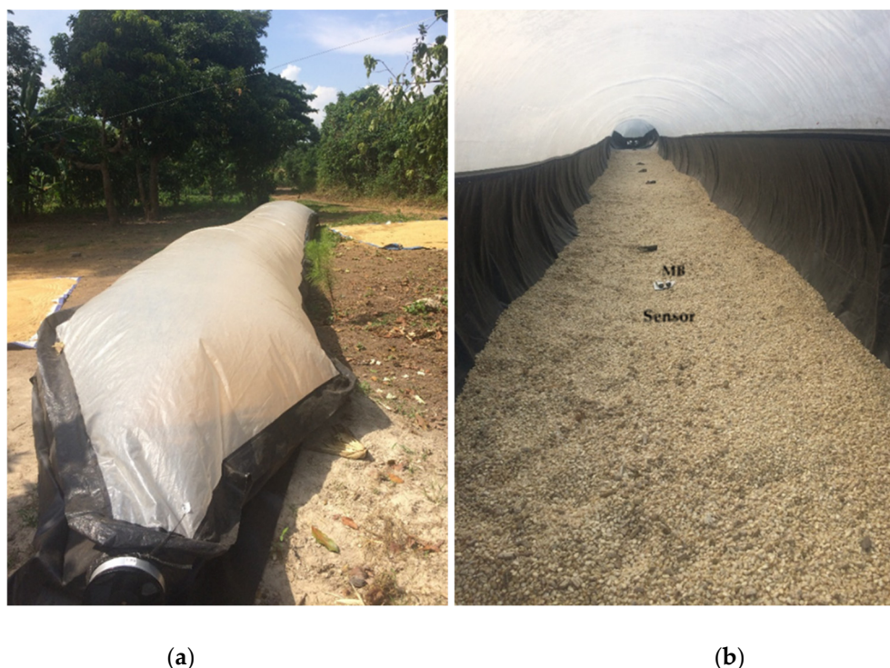
Figure 1. Inflatable solar dryer (ISD): (a) view from outside fully loaded with 1000 kg of maize and (b) inside view during the drying experiment showing the location of different sensors and mesh bags (MB).
