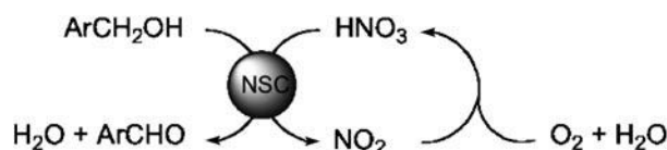
Figure 2-5 BzOH oxidation by \text{O}_2 and \text{HNO}_3 with NSC catalyst. Reprinted from ref. 56 with permission.
