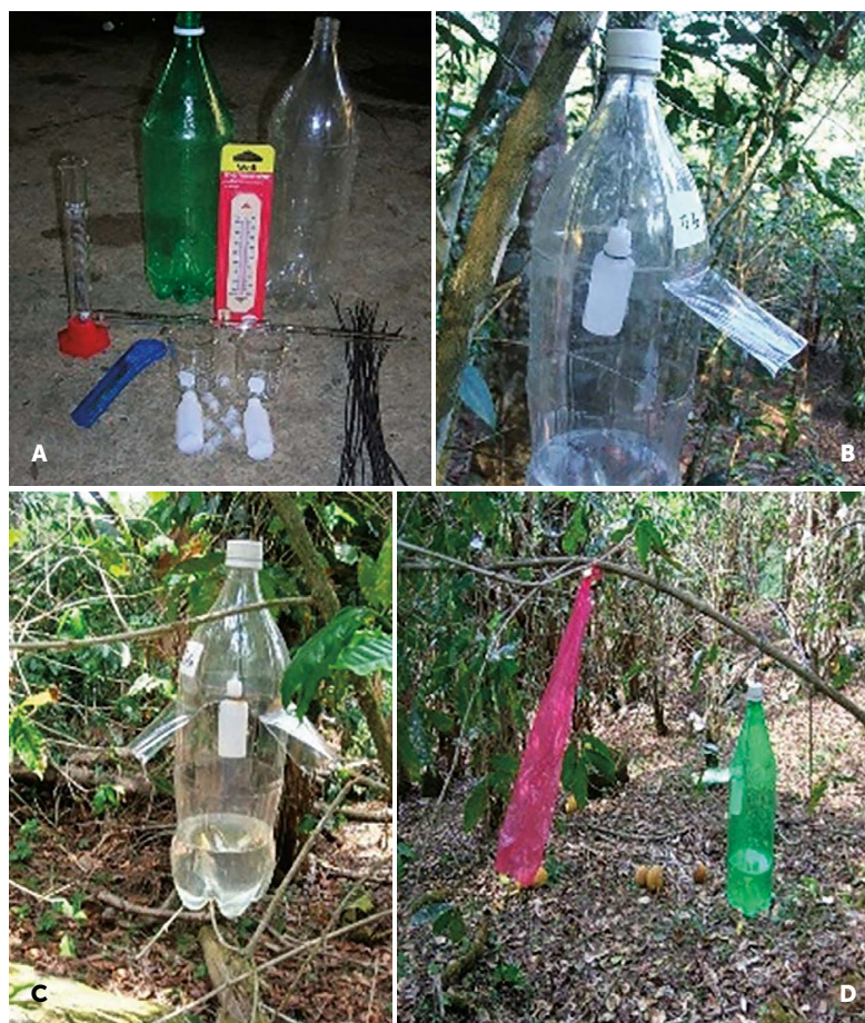
Figure 1. Traps to capture of H. hampei in El Paraíso, Guerrero, Mexico. A) Materials used; B) Trap with one window; C) Trap with three windows; D) Identification and placement of traps.
