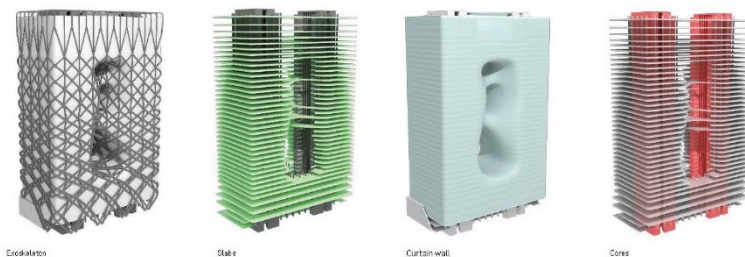
Figure 6.28. Rationalisation of the Morpheus building components: exoskeleton, floor slabs, curtain wall and cores. Morpheus Hotel , Zaha Hadid Architects, 2019.
