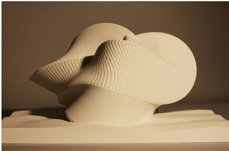
Figure 6.74. 3D printed shell prototype in polymethyl methacrylate (PMMA) with a rapid prototyping technique. Melika Aljukic et al., ARACHN[OL]OIDS (London: Architectural Association, 2013).
