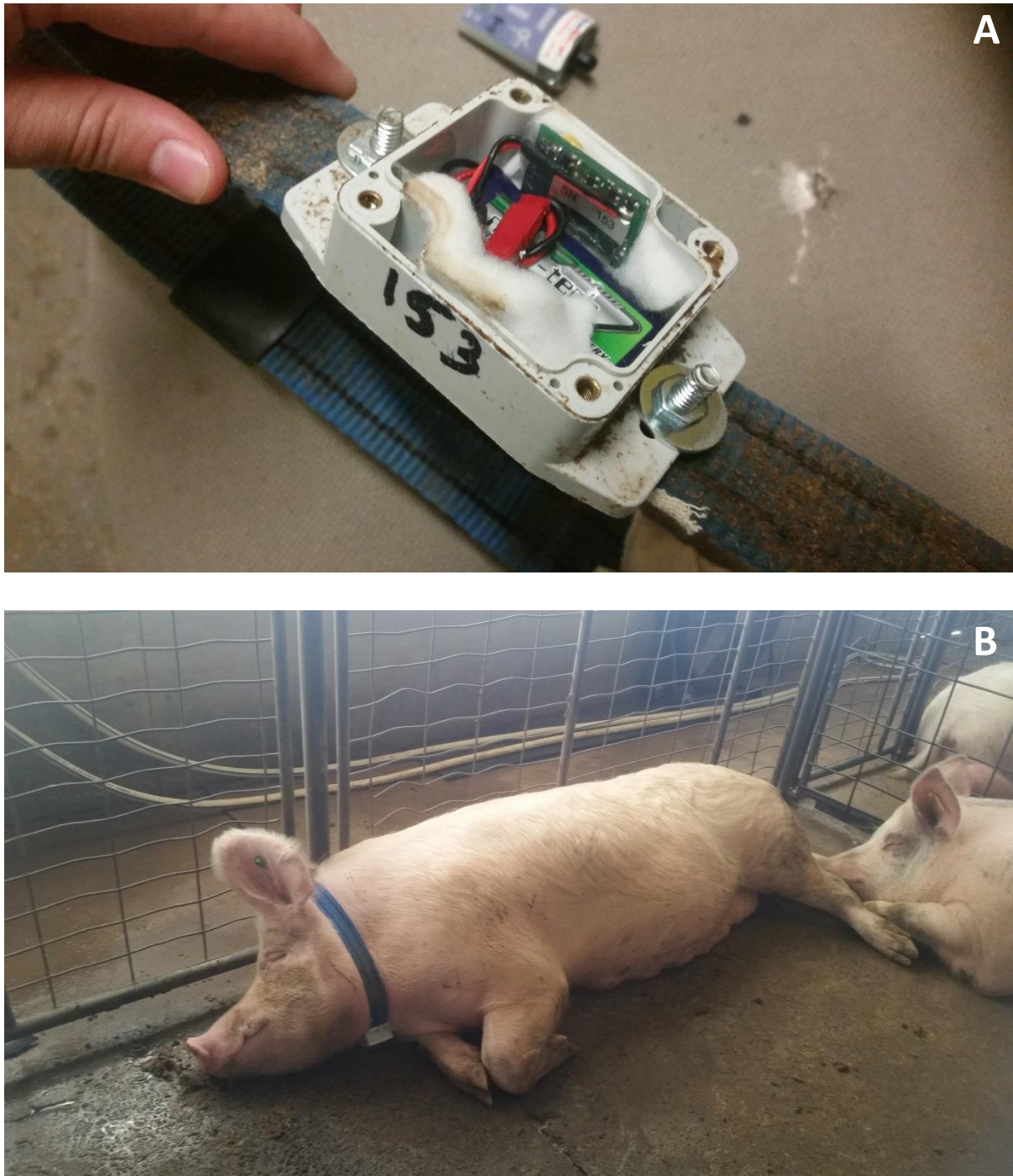
Figure 5.2. Panel A displays the arrangement of the battery and data motion logger inside the enclosure box mounted on the nylon collar. Panel B displays the placement of the enclosure box, on the ventral surface of the neck, when the collar is worn by the sow.
