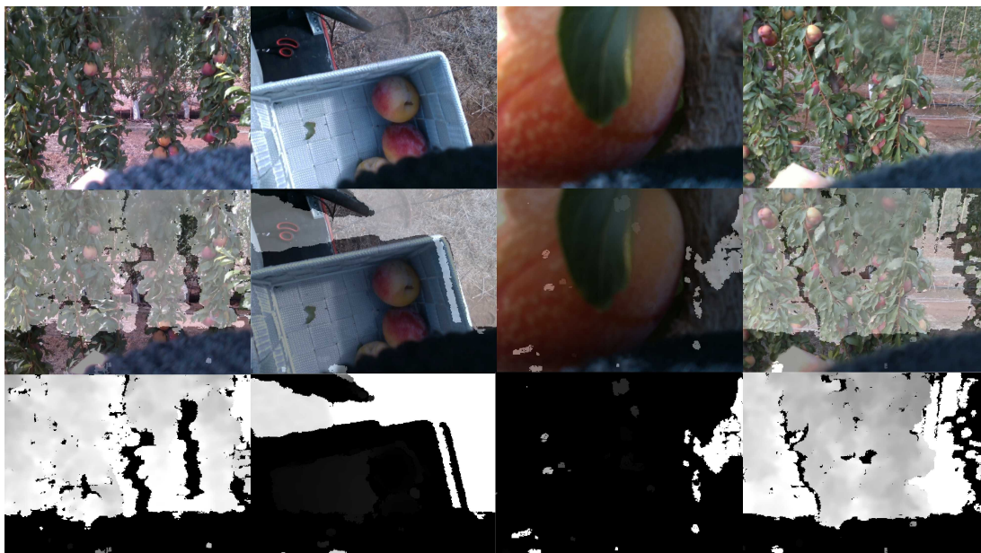
Figure 4.3 – Example RGB, RGBD overlay and depth images from the day dataset. Including effects specific to harvesting motion such as large illumination, object size and obscuration changes. Depth images shown after clipping is applied.
