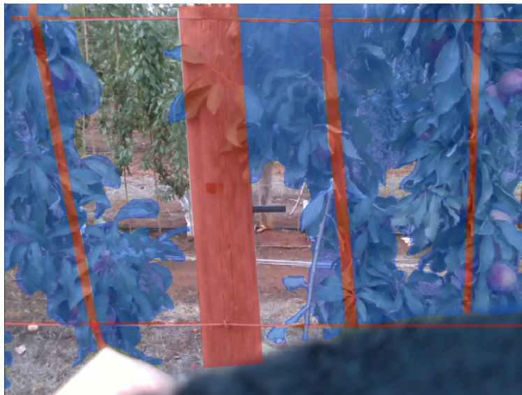
Figure 5.4 – Example frame with hard obstacles highlighted in red and soft obstacles in blue. Part of the gripper and one fingertip can be seen in the foreground.
