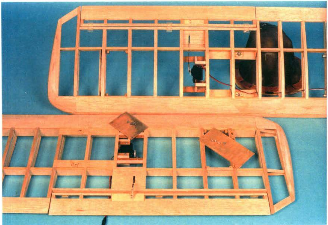
Figure B.18 Wing structure. Note: servo linkage to aileron; probe attachment points 4th rib outboard of servo; strut attachment points just after 2nd rib inboard of servo.
