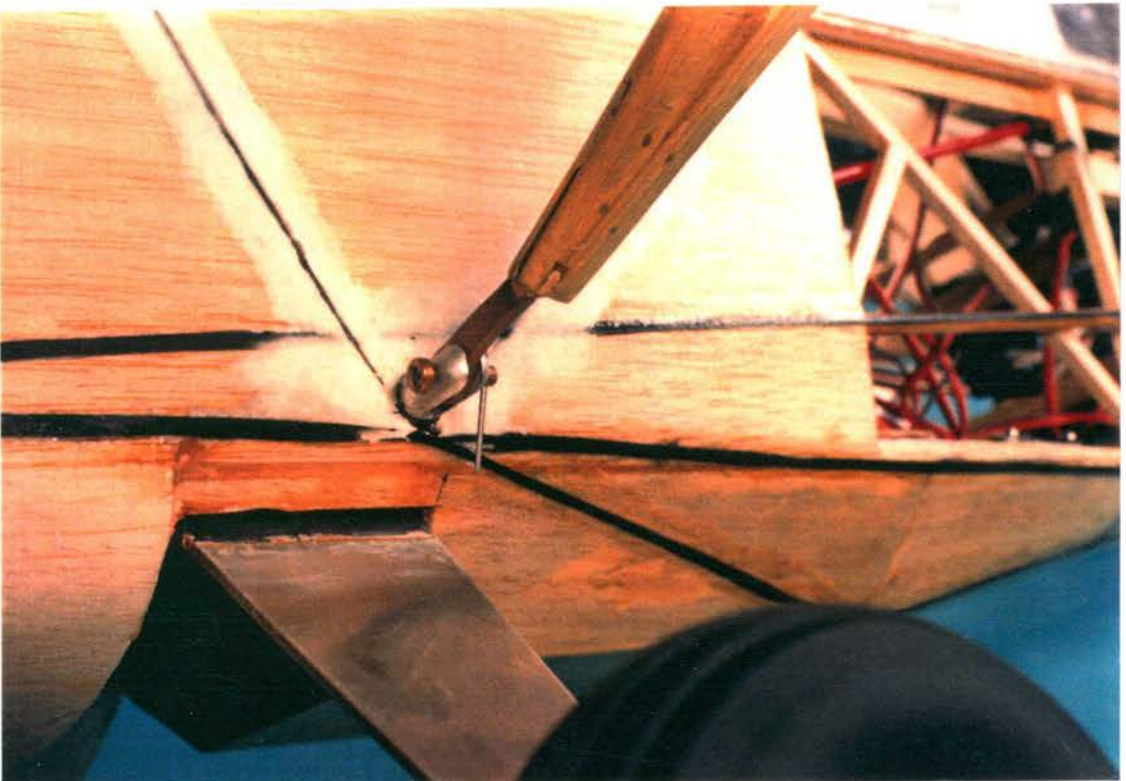
Figure B.20 Strut attachment point on fuselage.
