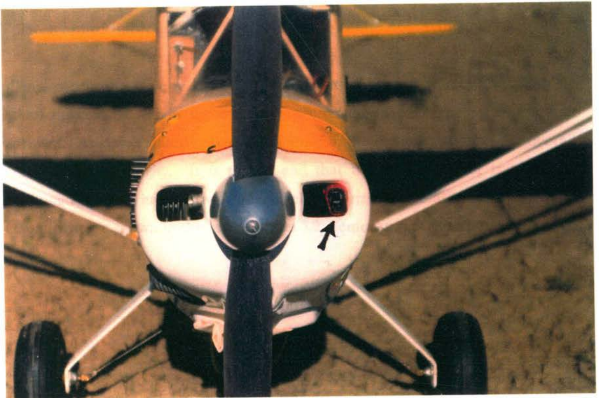
Figure 38 Location of engine speed sensor
