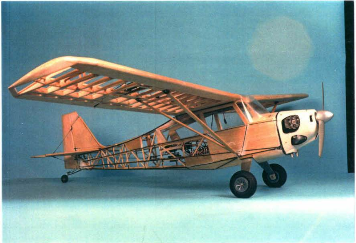
Figure B.7 Another view of KCEXP-2 before covering.
