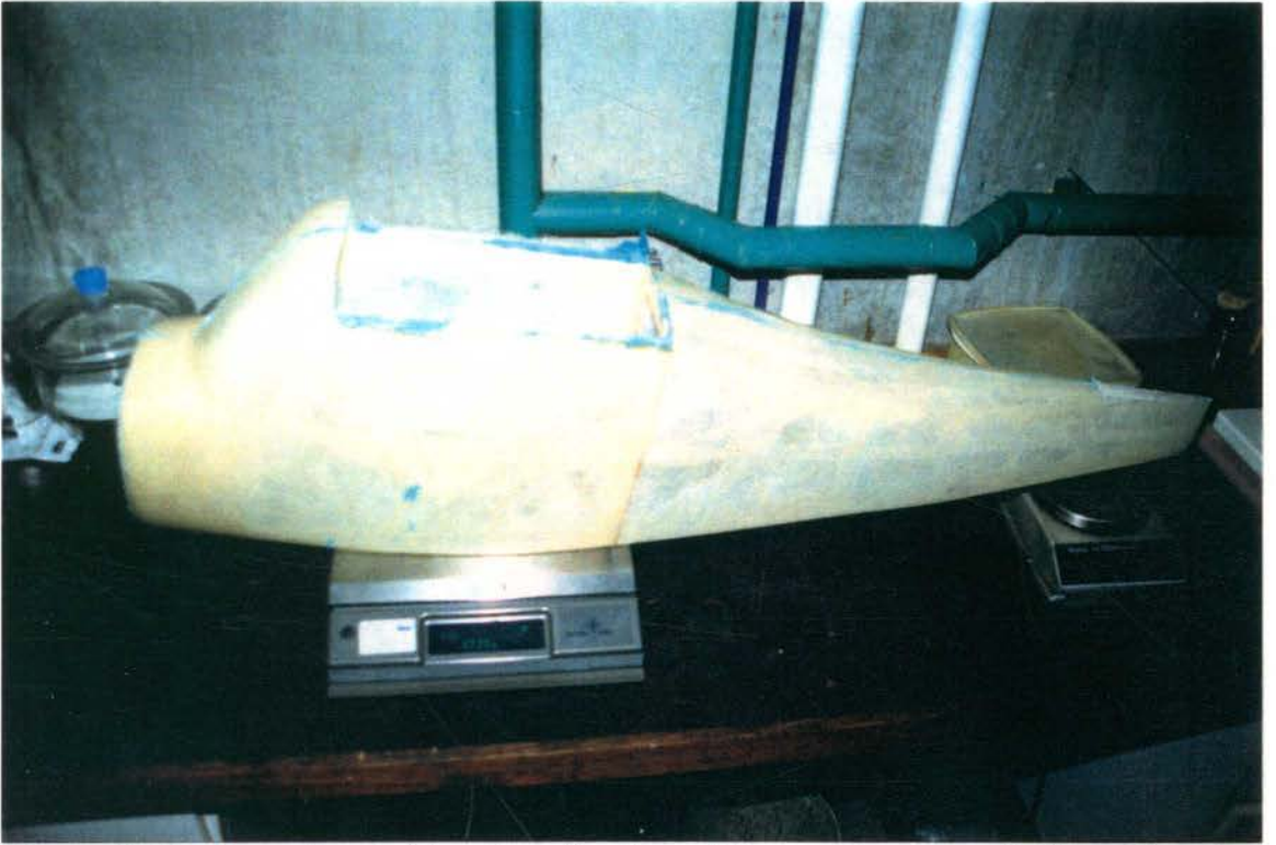
Figure B.39 Completed fibreglass fuselage fitted with plywood firewall and bulkheads - 1.739 kg. at this stage.
