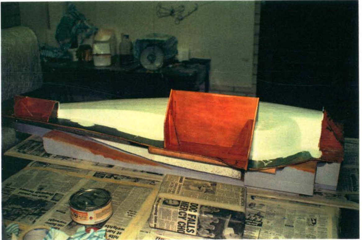
Figure B.31 White gel-coat applied for better surface finish.
