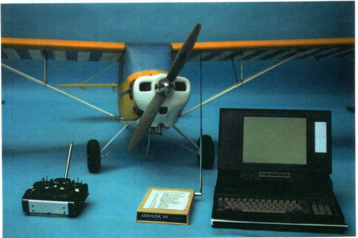
Figure C.8 KCEXP-3 with Aerolink-101 Telemetry receiver and JR PCM-10 command transmitter.
