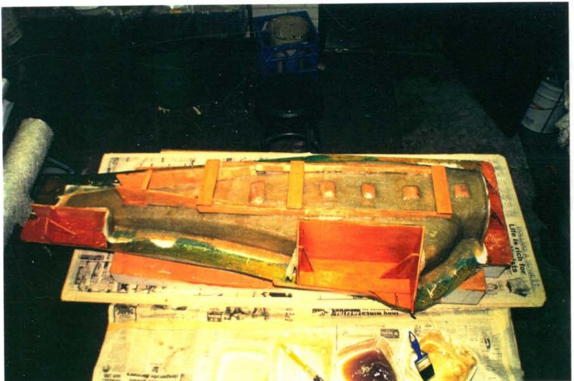
Figure B.32 Fibreglass half-mould complete with stiffeners.
