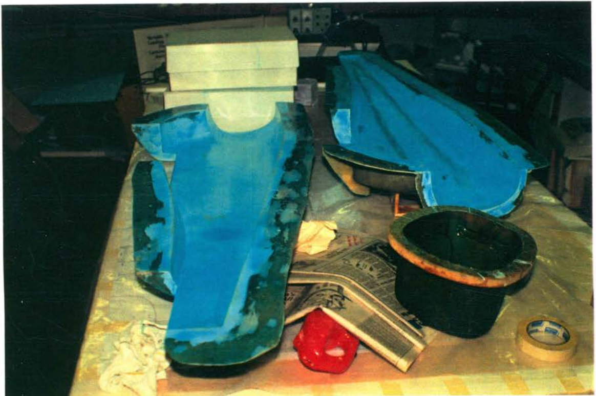
Figure B.36 Release agent applied. Note mould for cowl.
