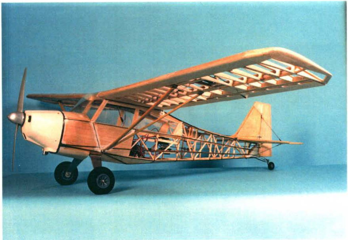
Figure B.6 KCEXP-2 - showing fiberglass cowl and carbon fibre reinforcements.
