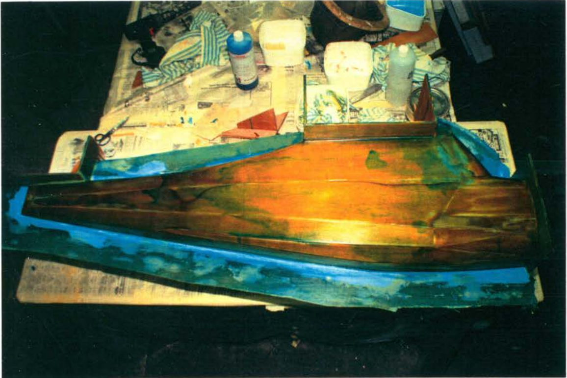
Figure B.30 Release agent applied.
