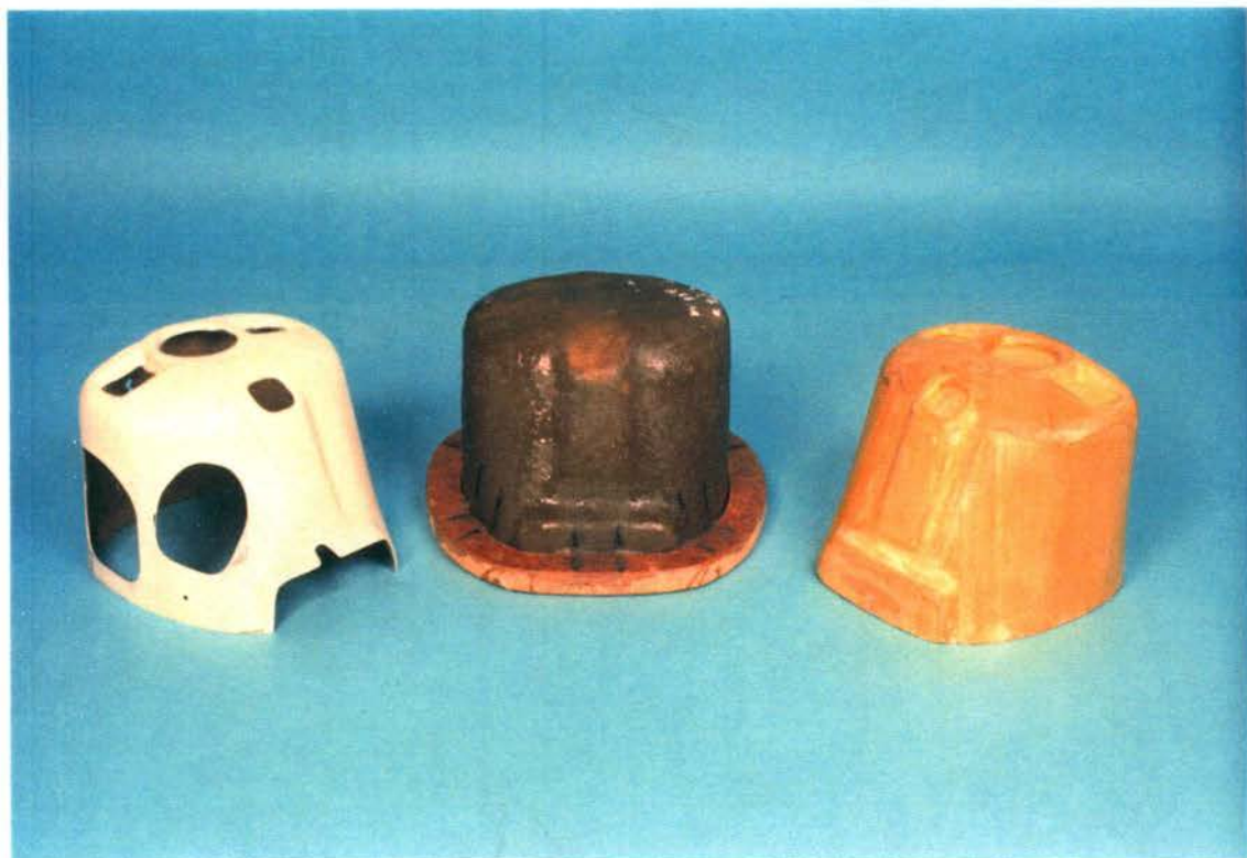
Figure B.11 Right - wooden plug of cowl; Centre - fiberglass mould; Left - finished fiberglass cowl.
