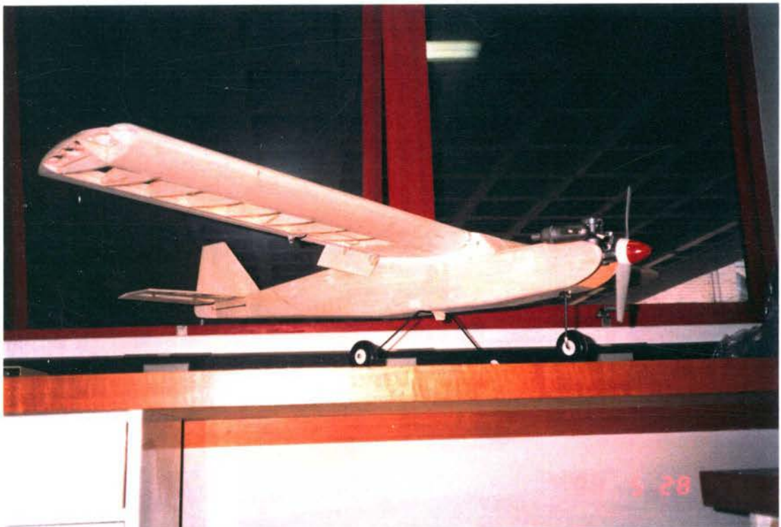
Figure B.2 KCEXP-1 - showing wing-fuselage assembly and flaps.
