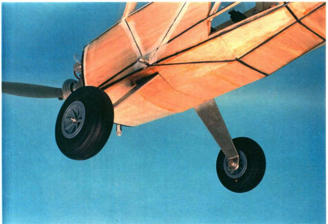
Figure B.14 Assembled main undercarriage. Note carbon fibre strips on fuselage.
