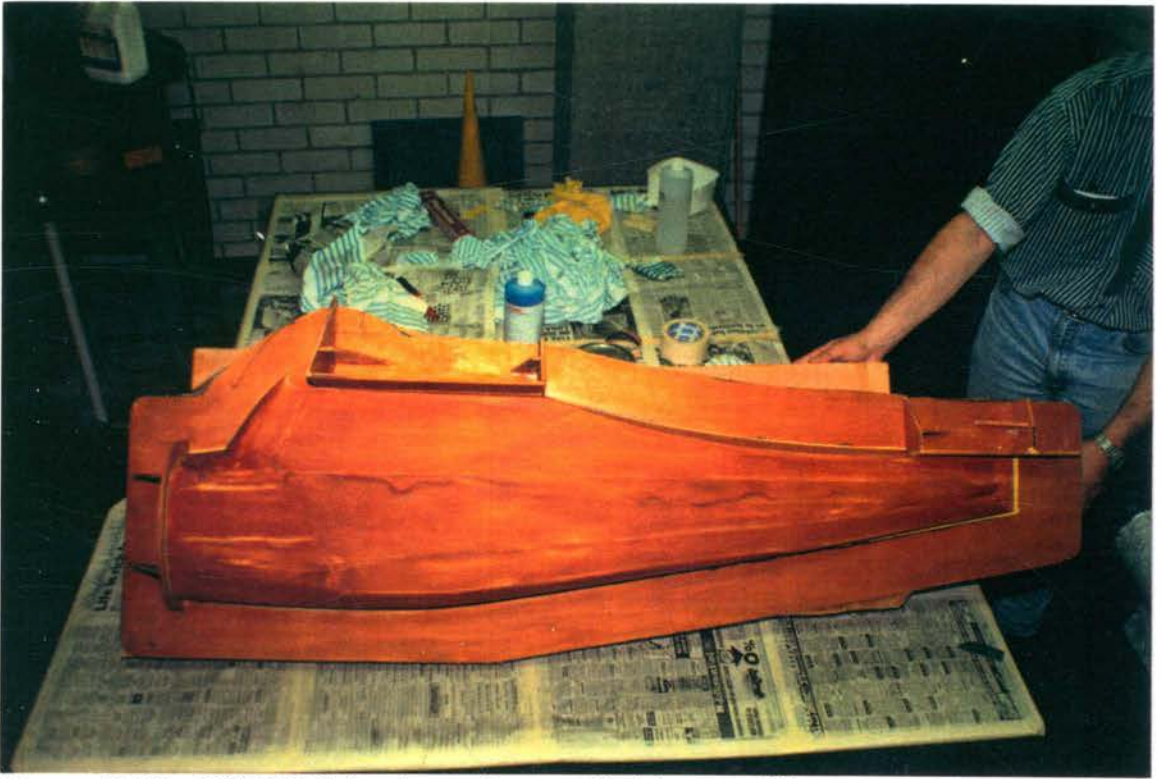
Figure B.29 KCEXP-3 fuselage plug readied for moulding.
