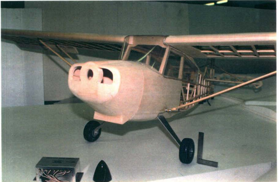
Figure B.5 KCEXP-2 - showing original wooden cowl.
