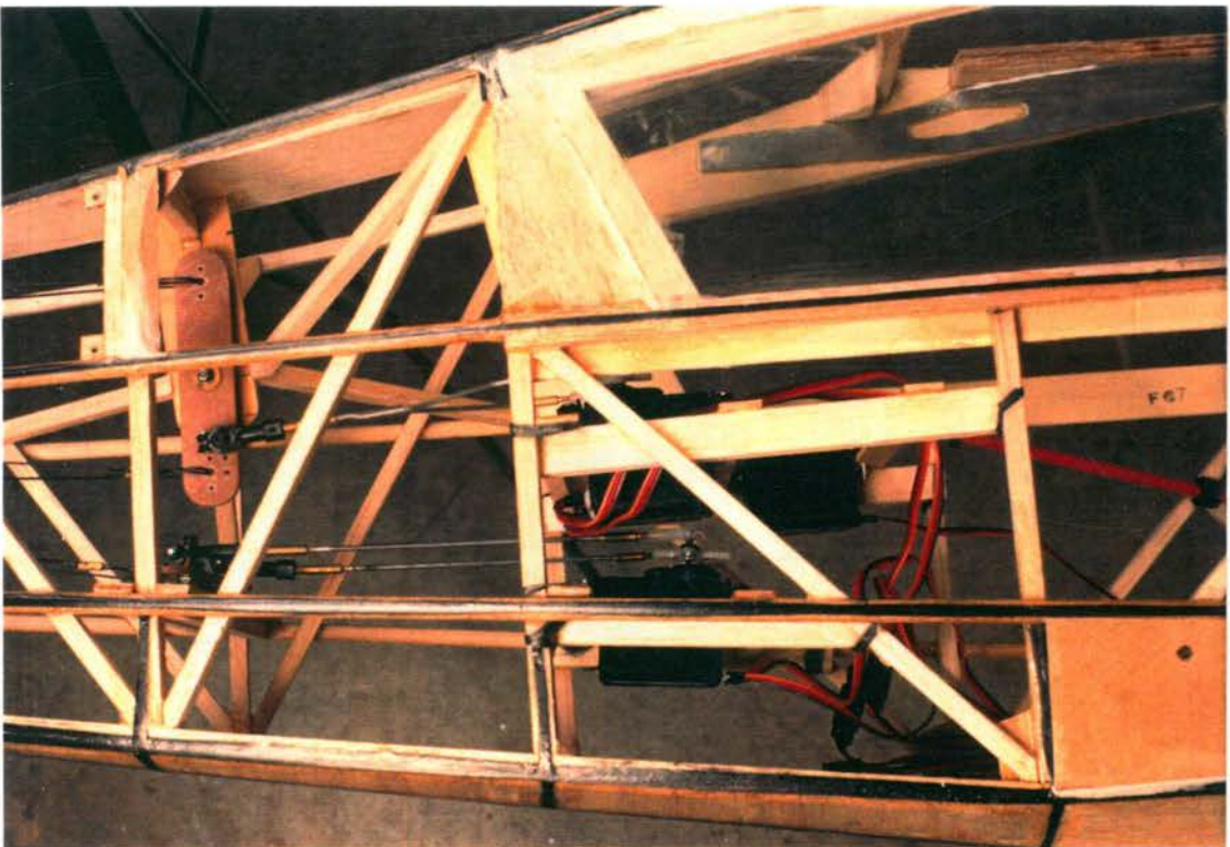
Figure B.24 Close-up of control linkage assembly.
