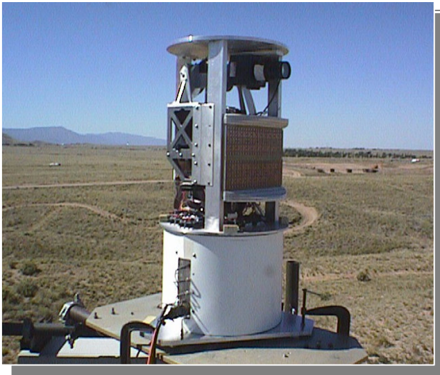
Figure 7: Advanced Exterior Sensor (AES) system integrates the three sensor technologies of thermal infrared imaging, visible light imaging, and microwave radar.
