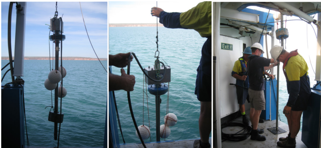
Figure 2.1. Coring method using a Vibecore-D (Speciality Products, USA) weighted vibrating head lowered from the CTD winch on the RV Solander.
