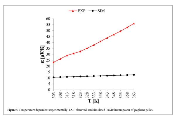
component while the phonon drag component contributes a little to the effective TEP [44]. Therefore, we can say that the linear increase in TEP indicates metallic diffusion behavior while the contribution by the phonon drag is negligible due to weak electron-phonon coupling [45, 46] in graphene pellet. The experimentally observed TEP is clearly following the predicted TEP.
