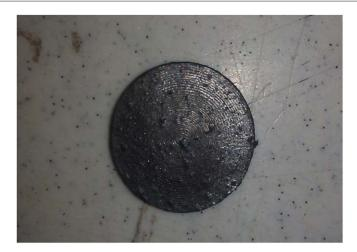
Figure 1. Graphene pellet.
