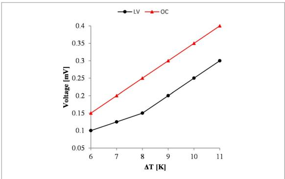
$\textbf{Figure 5.} \ \ Voltage-Temperature\ gradient\ relationship\ of\ the\ graphene\ pellet.\ OC\ represents\ the\ open\ circuit\ voltage\ while\ LV\ represents\ the\ voltage\ across\ a\ load\ resistor.$
