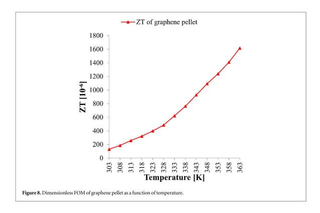
thermal conductivity could have resulted in high value of ZT for graphene pellet but this is not the case here as the electrical conductivity is very low which makes the power factor ( $\alpha^2 \times \sigma$ ) very small. In order to increase the FOM of the bulk-graphene, a further study is needed to increase the electrical conductivity while still keeping the thermal conductivity to low values.
