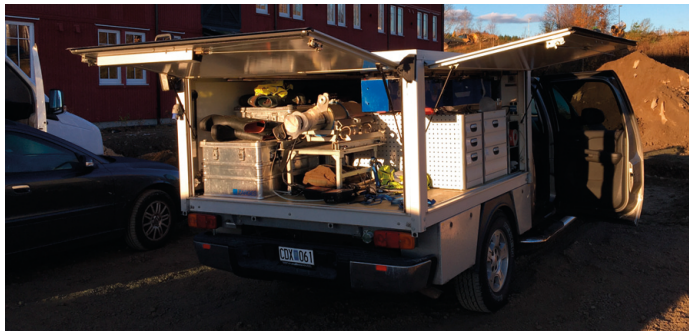
Fig. 19. An image of the open service bed portion of the mobile gamma spectrometry vehicle used throughout the thesis. The 123% HPGe detector with a cryostat can be seen in the back of the service bed, with the sensitive medium of the detector pointing to the back of the vehicle. The two blue boxes in the top of the right side of the service bed are the 4l NaI(Tl) detectors. The GNSS receiver is mounted on the roof of the cabin of the car. Figure from paper II.
