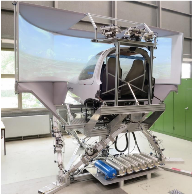
Figure 1. The platform manipulator as a part of the flight simulator for Diamond DA42 Twin Star aircraft (Institute for System Dynamics, University of Stuttgart, Germany) [10].
