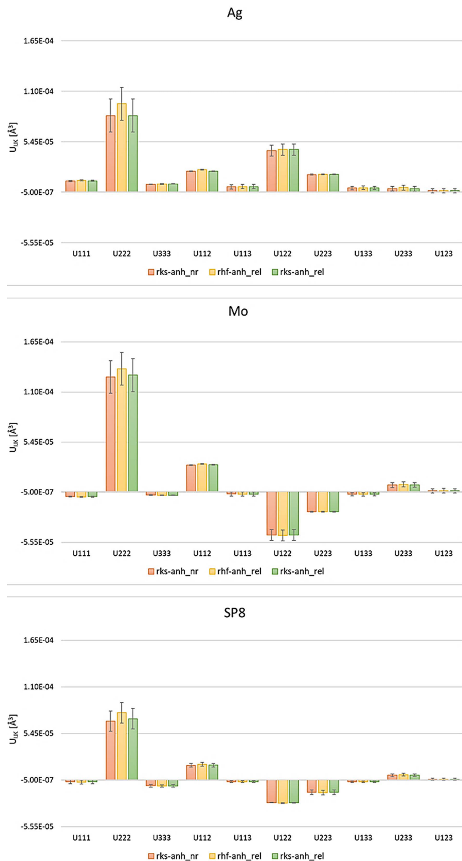
Figure 5 Plot of the numeric values of the significant third-order GC coefficients within three e.s.d.s for Ag, Mo and SP8 data for HARs at different levels of theory.
