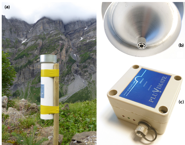
Figure 2. Drop-counting rain gauge used for rainfall measures. The Pluvimate is set up vertically, between 0.8 and 1.2 m above the ground level (a). A tip at the end of the funnel (b) creates a calibrated drop of water that falls on the sensor, (c) which counts and records the number of drops during a given amount of time.
