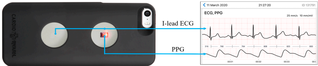
Figure 1. Characteristics of CardioQVARK device. On the left side , there is the electrode for I-lead ECG registration and on the right side the monitor for photoplethysmography PPG. The device is shown together with an example of the presentation of the recording.
