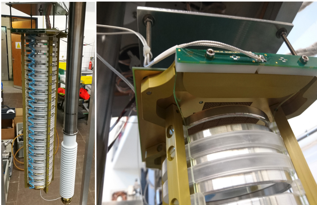
Figure 5. Photographs of the pixel demonstration TPC at Bern, with the HV feedthrough. A close-up of the light collection system shows wavelength shifting fibers coupling SiPMs to the TPB-coated light guides.
