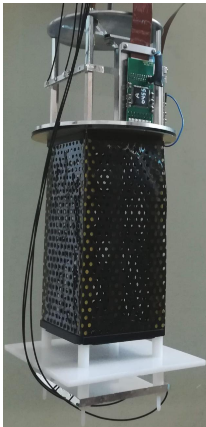
Figure 3. The Bern field-shell demonstrator LArTPC. The field-shell and cathode are made from \sim 50 \mu\text{m} resistive kapton foil. For this test, the field-shell was perforated to allow the purification of the LAr within the active volume. The Time Projection Chamber (TPC) has a 7 \text{ cm} \times 7 \text{ cm} footprint and a 15 cm drift length. A bias of up to -23 \text{ kV} was applied to the cathode to generate a 1.5 \text{ kV cm}^{-1} drift field [34].
