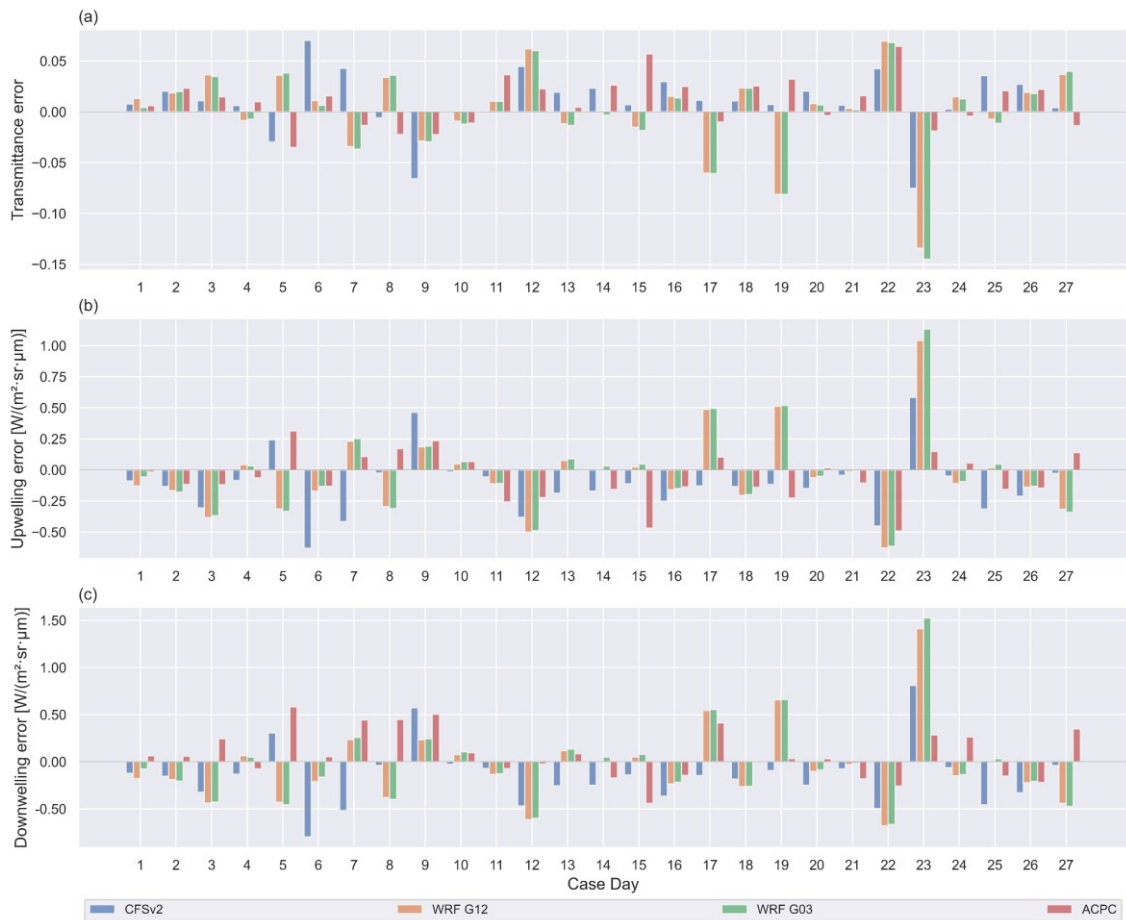
Fig. 5. Errors in the estimation of (a) atmospheric transmittance, (b) upwelling radiance, and (c) downwelling radiance from the different profiles for each case day.
