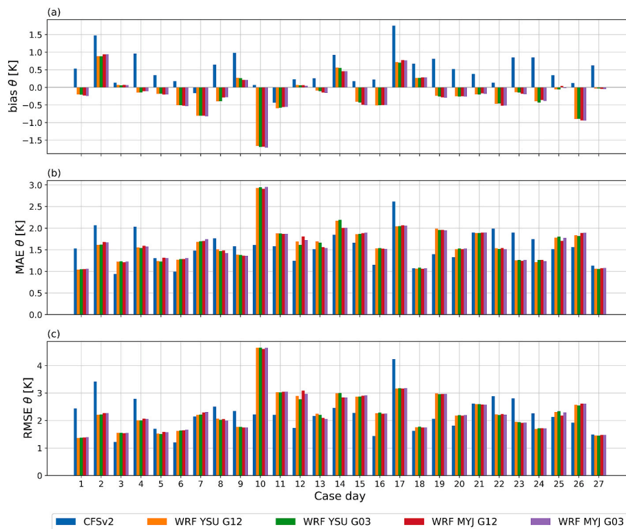
Fig. 5. Statistical metrics: (a) bias, (b) MAE, and (c) RMSE; over the case days for \theta .
