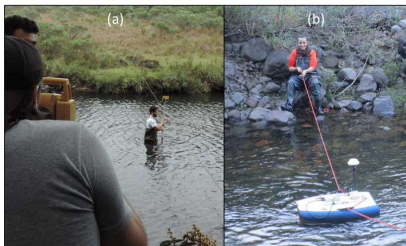
Figure 2-2 – Field survey and measurement: (a) morphometric parameters by using a total station; and (b) discharge by using ADCP (Source: elaborated by the authors)
