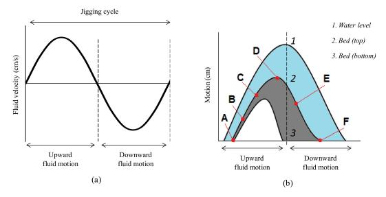
**Figure 5.** Illustration of (a) fluid velocity and (b) fluid and bed motion along a sinusoidal pulsation cycle in a jig. The points A to F represent the behavior of the jig bed at different moments within the cycle (see Figure 6).
