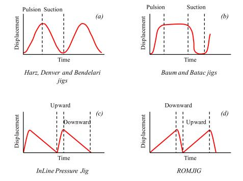
**Figure 9.** Typical pulsation diagrams of different jigs. (a) sinusoidal, (b) trapezoidal, (c) "saw-tooth" with rapid upward, and (d) "saw-tooth" with rapid downward.
