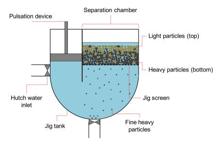
**Figure 1.** General scheme of a jig (front view).
