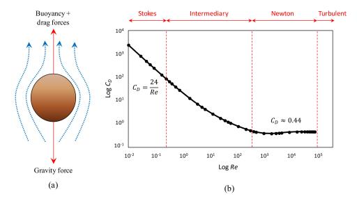
**Figure 7.** (a) Forces acting on a spherical particle in a fluid; (b) drag curve for motion of a sphere in a fluid. The curve was plotted based on the model of Haider and Levenspiel [61], see Equation (9).
