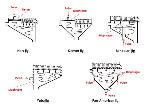
Figure 3. Scheme of some piston and diaphragm-type jigs (adapted from Sampaio and Tavares [8]).
