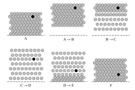
**Figure 6.** Jig bed motion over a pulsation cycle. The displacement of the particle colored in black represents the variation in the position of a dense particle within a bed of light particles.
