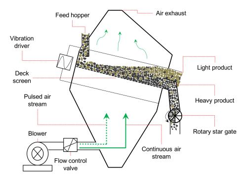
Figure 4. Basic scheme of a dry jig.
