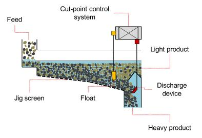
Figure 2. General scheme of a jig (side view).
