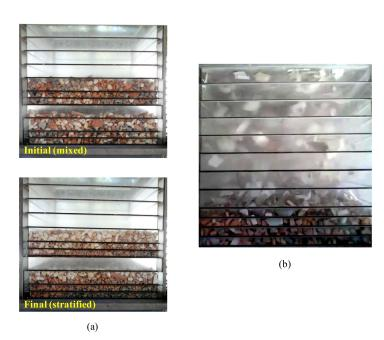
**Figure 13.** (a) Placement of a second bed in the container of a batch dry jig. (b) Snapshot of testing the removal of organic contaminants from a mixture of aggregates.
