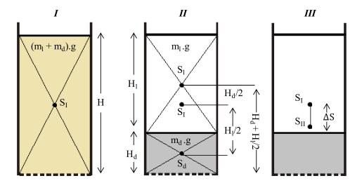
**Figure 8.** Position of the center of gravity in a binary mixture of particles with different densities. (I) homogeneous mixture, (II) perfect stratification, (III) lowering of the center of gravity. Adapted from Mayer [68] and Sampaio and Tavares [8].
