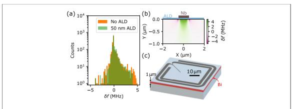
**Figure 1.** (a) Histogram showing simulated strain-induced frequency shifts in silicon underneath a 1  $\mu$ m wide, 100 nm thick Nb wire at 4 K with and without a 50 nm ALD layer. (b) A map of the strain induced shifts which are binned to generate histograms in (a). The ALD and Nb wire are shown to scale on the top of the panel. (c) A schematic of the devices used in this work showing the layout of the superconducting resonator atop an implanted substrate.
