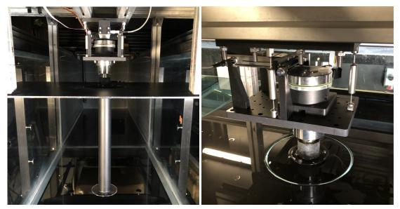
(a) Cylinder mounted to the carriage.(b) Motor mounted to the force balance.Fig. 3.9 Experimental set-up in the water tank.
