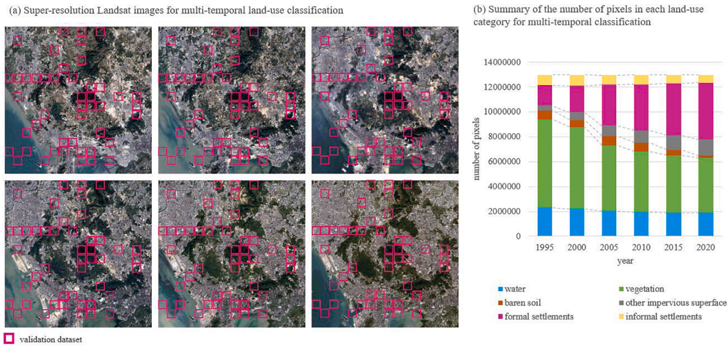
Fig. 4. Dataset settings for multi-temporal land use classification tests: (a) super-resolution Landsat images (b) number of pixels for each land use category.
