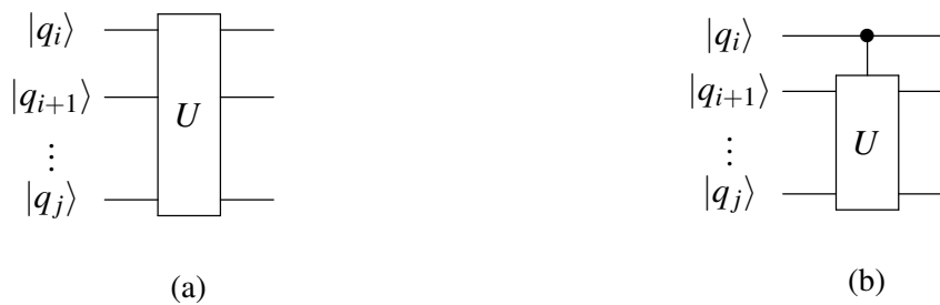
Fig. 1.4 a) Quantum gate corresponding to a general unitary operator U . b) Quantum gate corresponding to a general unitary operator U controlled by the state of qubit i .
