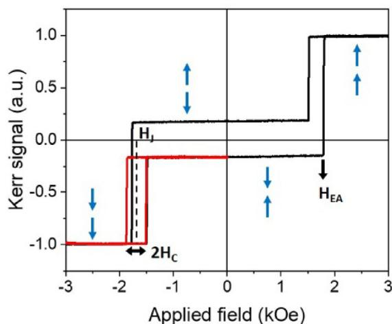
Figure S1 Diagram showing how the magnetic variables are obtained from easy axis major (black) and minor (red) hysteresis loops of a thin film. The blue arrows represent the direction of magnetisation of each of the CoFeB layers.
