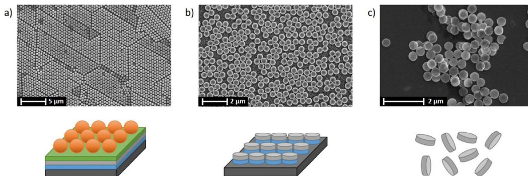
**Figure S3** Three key steps of the new nanodisc fabrication method: (a) the plasma ashed PS bead lithography mask; (b) ion milled nanodiscs, on chip, after the removal of the mask; and (c) nanodiscs that have been lifted off and redeposited for imaging. Each step is depicted by a schematic (taken from Fig. 2) and a corresponding SEM image.
