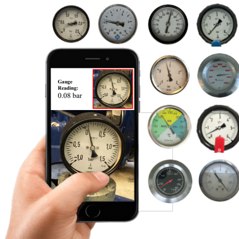
Figure 1. Our system runs in real-time on mobile phone and is capable of transcribing unseen analogue gauges to a very high accuracy. The system is trained purely from synthetic data yet transfers very well to real world meters and is robust against the huge appearance variation in real world gauges due to bezel types, pointers and background scales.
