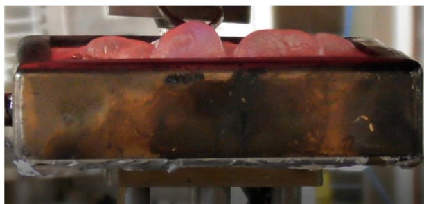
Figure 6. The behaviour of the coating based on starch acting as a blowing agent, heat flux 35 \text{ kW/m}^2 , 20 s before the ignition.
