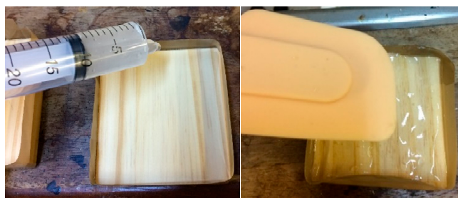
Figure 1. The application of starch-based coatings onto the surface of Taeda pine wood samples.
